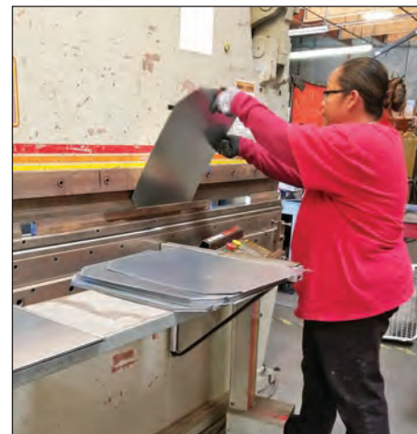
Allelea Cabiles, now a third-year apprentice and member of Local 104, bends metal sheets as a pre-apprentice to make storage bins for hardware for F.W. Spencer in Brisbane.
